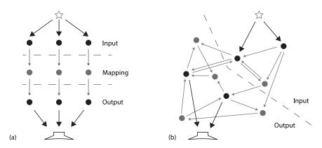
**Figure 3** Instrument structure according to (a) Wessel vs. (b) a more open structure with non-hierarchical constraints. Note that the explicit mapping shown in (a) is blurred in (b) due to system-inherent feedback.
