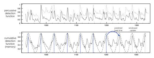
**Figure 1** Predictive beat tracking using the cumulative detection function on a percussive detection function. The percussive filtered detection function is shown in bold and the standard onset function using complex spectral difference is shown as a dotted line.
