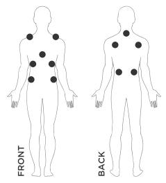
Figure 7 FSR's positions on the mannequin.
