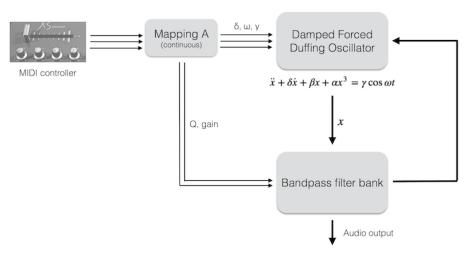
**Figure 1** Interface 1. A damped forced Duffing oscillator coupled with a bank of linear resonators. The user interacts with the system via three MIDI controls.
