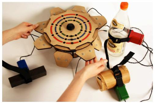
**Figure 2** Moving the flaps on the Drum Duino control panel with all three actuators in view
