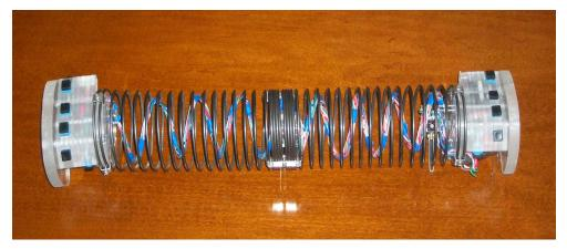
**Figure 1** The Sonik Spring can be compressed, expanded, shaken, twisted or bent in any direction, prompting the user to combine different types of intricate manipulation.
