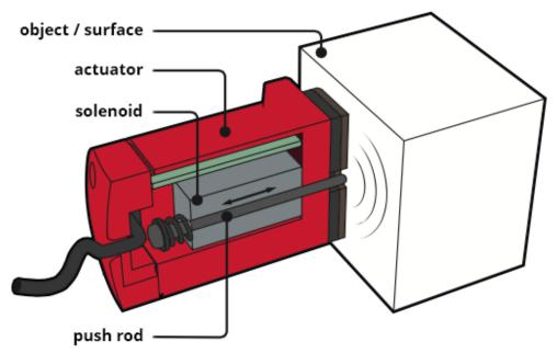
Figure 1 Overview of the actuator, pushrod and solenoid
