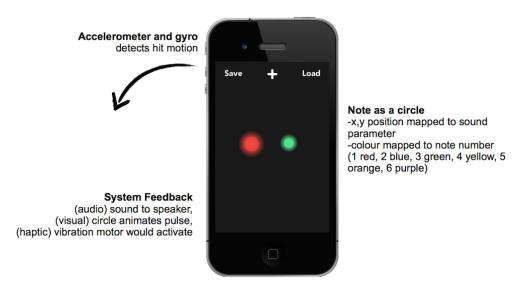
Figure 3 The instrument's user interaction design
