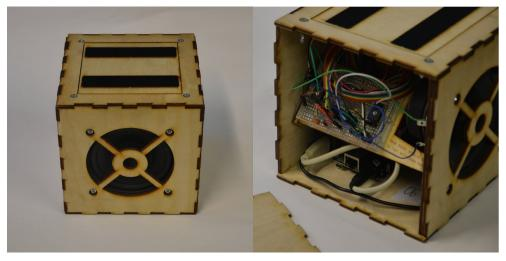
**Figure 2** On the left: shot of the of the D-Box, showing the 2 sensors and the speaker. On the right: a detail of the matrix.
