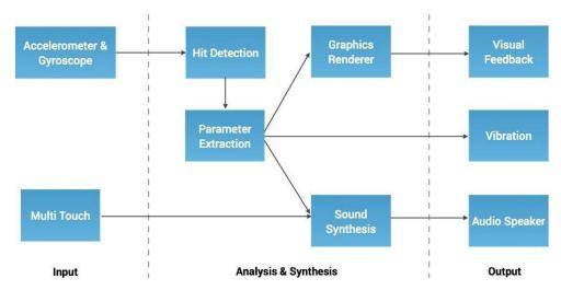
Figure 4 System architecture design
