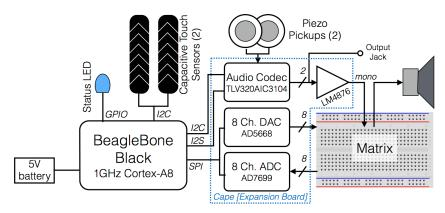
**Figure 1** Hardware for the D-Box. Hacking is focused on changing the matrix, a bread-board accessible through the side of the box, though other elements of the instrument can also be altered.
